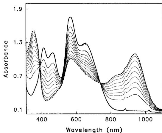
**Figure 2.** Spectral changes attendant upon the reduction of  $4.5 \times 10^{-5}$  M dication  $1^{2+}$  (—) to its cation radical  $1^{+•}$  (---) by incremental addition of  $1.8 \times 10^{-3}$  M **1** in dichloromethane at 25 °C.
