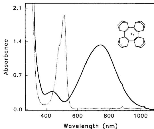
**Figure 3.** The UV-vis absorption spectrum, of cyclooctatetraene cation radical  $8^{+•}$  (—) generated by treatment of 0.3 mM **8** in dichloromethane with 1 equiv of [MA<sup>+</sup> SbCl<sub>6</sub><sup>−</sup>] (---) at 25 °C.
