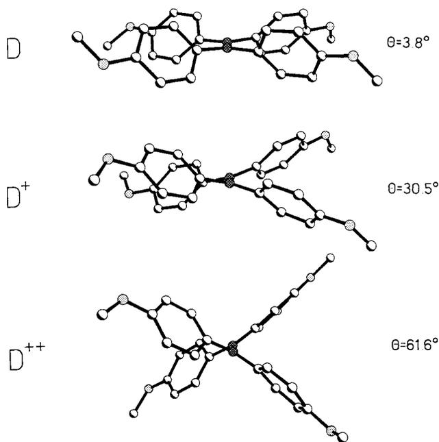
**Figure 8.** Linear increase in the dihedral (ethylenic) angles  $\theta$  in tetraanisylethylene (top), its cation radical (middle), and its dication (bottom). The latter shows the inequivalency of An<sub>1</sub> and An<sub>2</sub> in the dication.
