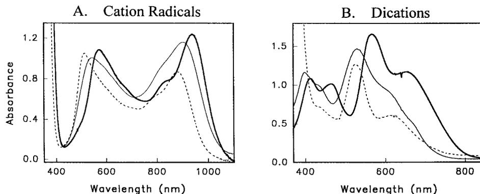
**Figure 1.** UV-vis absorption spectra of (A) the cation radical and (B) the dication from the oxidation of tetraanisylethylene **1** (—), tetratolyethylene **2** (---), and dianisyliditolyethylene **3** (- - -) with 1 and 2 equiv of  $[\text{EA}^{+\bullet} \text{SbCl}_6^-]$ , respectively, in dichloromethane at 25 °C.
