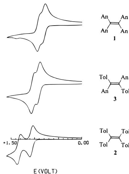
**Figure 5.** Cyclic voltammograms of 5 mM tetraarylethylenes **1**, **2**, and **3** (as indicated) in dichloromethane containing 0.2 M tetra-*n*-butylammonium hexafluorophosphate at a scan rate of  $\nu = 200 \text{ mV s}^{-1}$  (25 °C).
